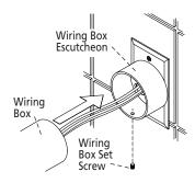
Fig. 2: Disconnectiom of Wiring Box
