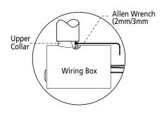
Fig. 4.1: Mounting of Towel Warmers with plastic brackets
